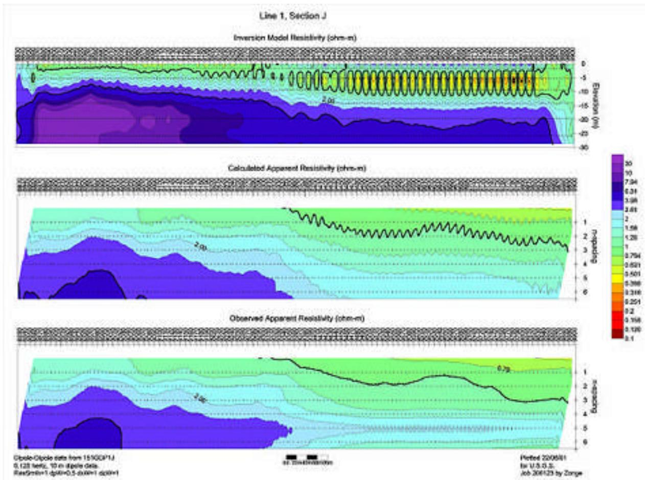
**Figure 7.** Cross section /pseudosection triad for Line 1j. This section corresponds to the last profile in Figure 10. Bottom segment is observed (raw) data plotted against dipole number on the vertical axis; middle pseudosection is calculated apparent resistivity, and top section is the inversion modeled depth/resistivity layered model.
