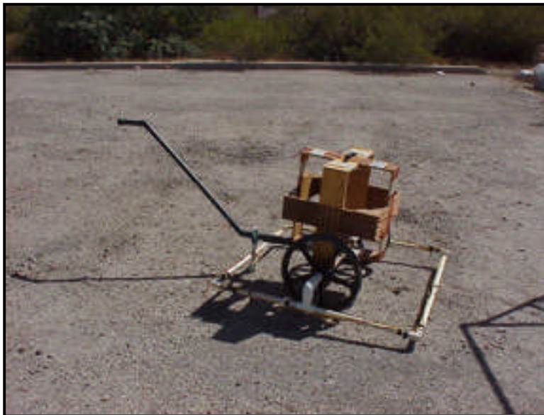
Figure 9: Experimental fast TEM antenna system for conducting simulated field experiments. The system consists of a 1m x 1m transmitter antenna and a 3 orthogonal 1/2m x 1/2m receiver antennas.
