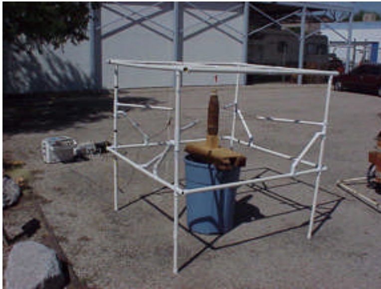
Figure 8: 5' x 5' Helmholtz transmitter antenna used for characterization measurements on large targets.
