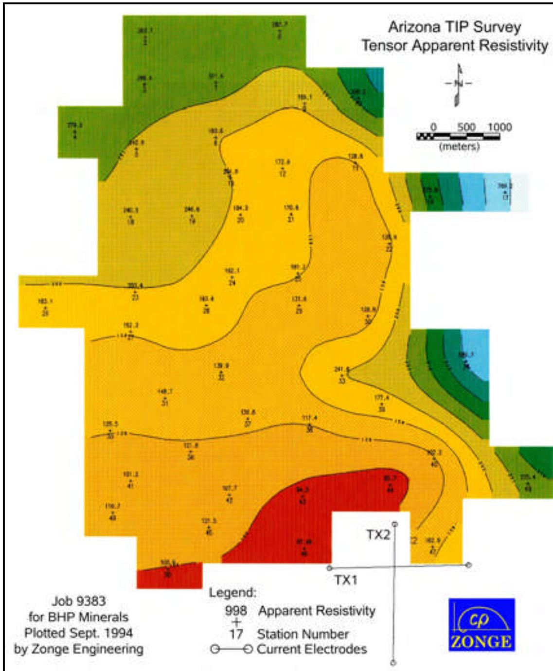
Figure 7: Tensor TIP "Resistivity" (TX1 & TX2)
