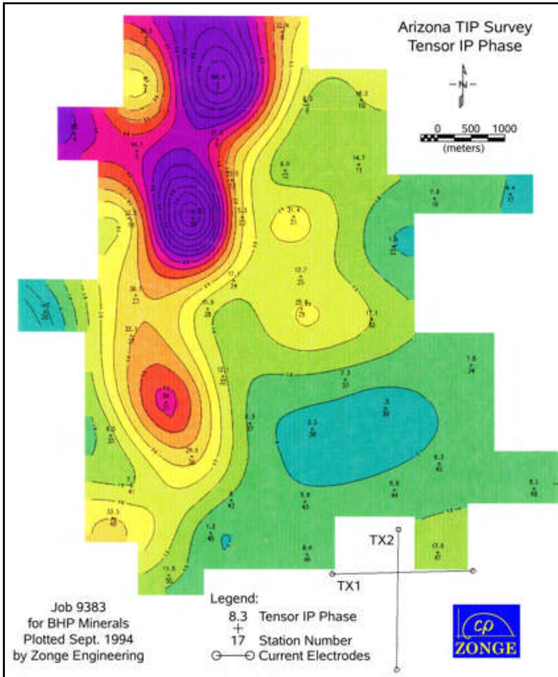
Figure 6: Tensor TIP "IP" (TX1 & TX2)
