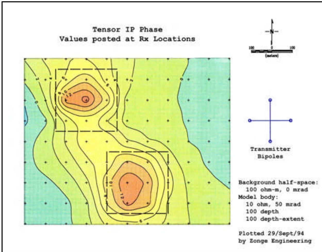
Figure 13: Two Body Tensor TIP Phase Model
