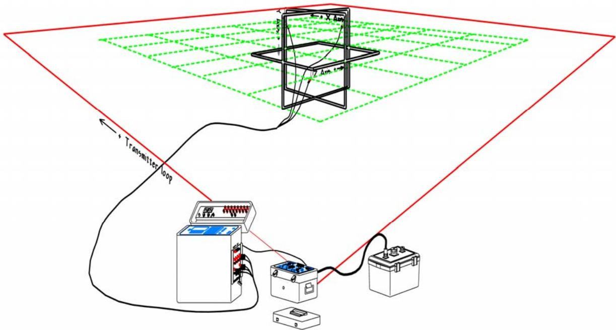
**Figure 1:** Basic setup of the NanoTEM system (GDP-32, NT-20, and NT Battery) using the three axis receiver loops. Usually a grid of six one meter by one meter stations is read within the each transmitting loop.
