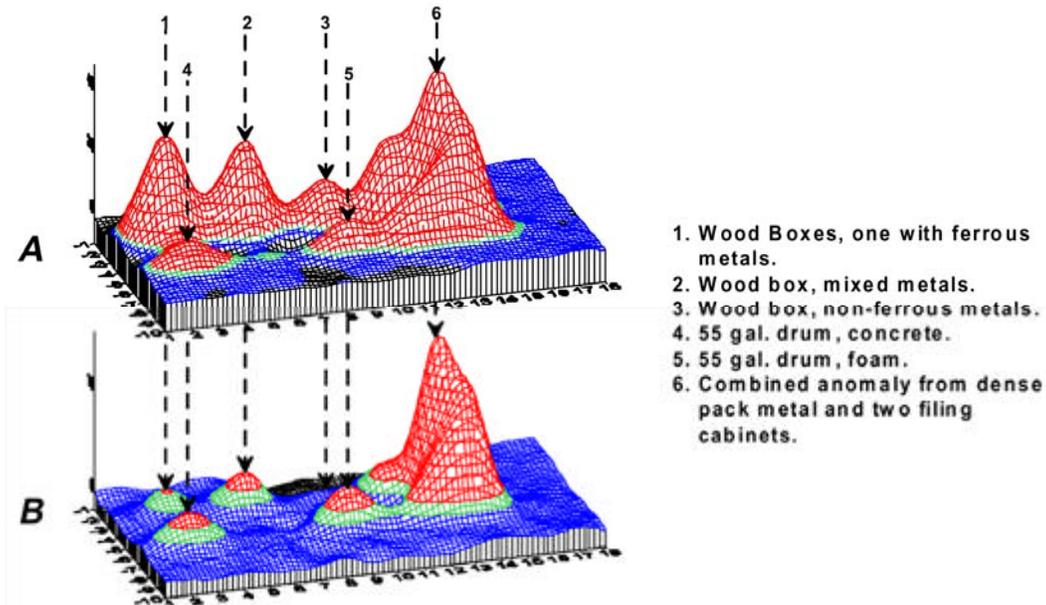
**Figure 2:** NanoTEM results over the Calibration Cell.
