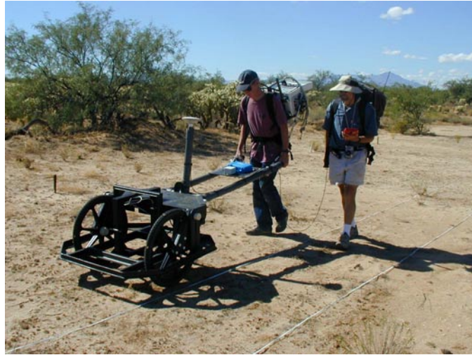
Figure 1: A cart-mounted Dynamic NanoTEM (DNT) system configured with a 1 by 1 m horizontal transmitter loop and three 0.5 by 0.5 m receiver loops arranged to measure x, y and z-component secondary magnetic fields. The smaller loops are optimal for detecting shallow objects at depths of 2 m or less.
