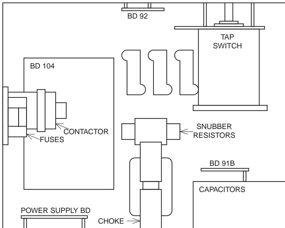
Figure 8. GGT-10, Contactor Side
