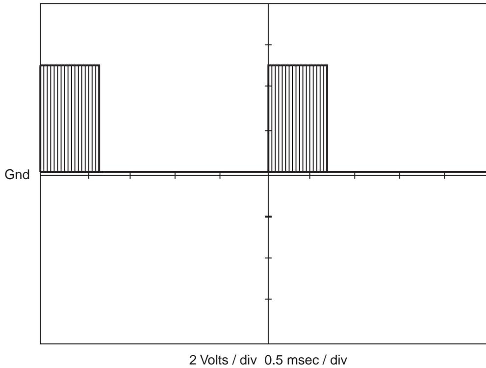
Figure 14. SCR Driver Waveform 38.4 KHz Burst
