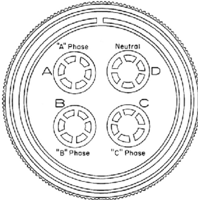
Figure 16. Power Cable, Military Plug, Transmitter end.
