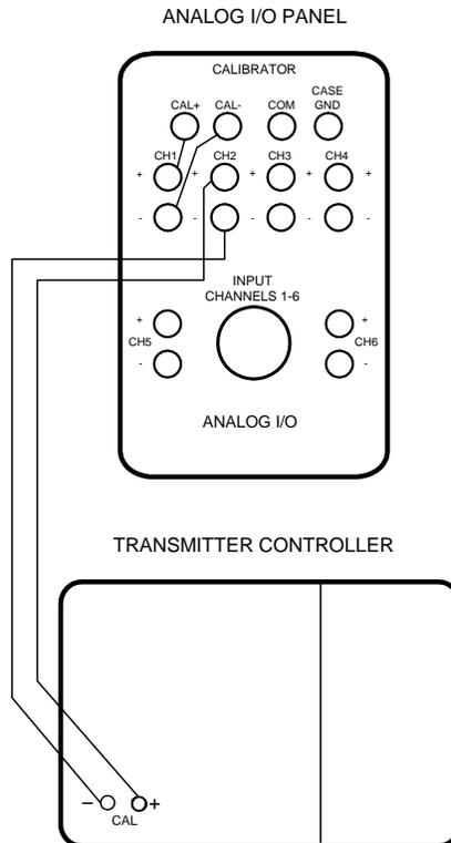
Figure 6.4(b) - Wiring for verifying synchronization to a large case GDP-32
