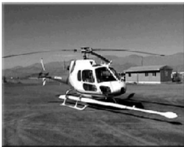
Figure 7-4. Fugro Airborne Survey's helicopter-borne stinger mounted magnetic sensor system (courtesy of Fugro Airborne Surveys).
