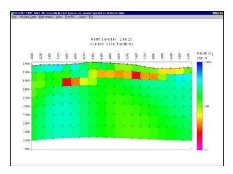
Re-running the inversion with gradient constraints cut around the low resistivity area, lets RSCS2D introduce a sharp offset between low resistivity and surrounding higher resistivity host material. Here, I have used **View | Zoom Rectangle** to select a detailed view of the model section.
