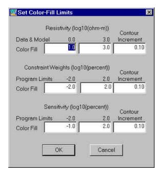
SCS2D's set color-fill limits dialog box includes fields for editing resistivity color-fill limits in units of log10(ohm-m). Constraint weight and model sensitivity color limits are also in log10 units. SCS2D saves color-fill limits in \*.MTM files, so that they don't have to be reset when you reopen an existing model file set.
