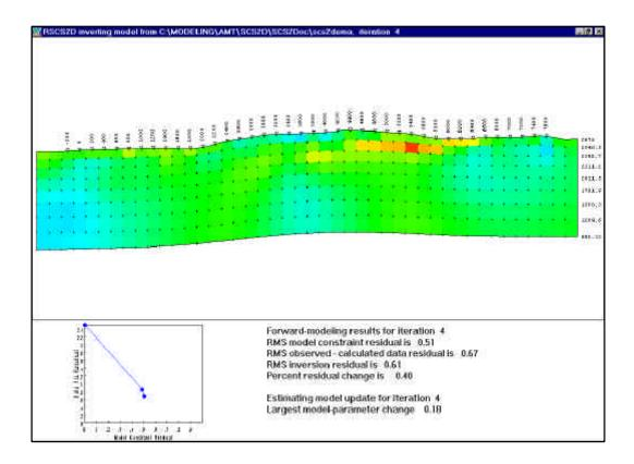
RSCS2D plots the inversion model section across the top two-thirds of its window. Scrolling text describing the inversion's progress is shown on the lower right quarter of the window and a plot of model-constraint residuals versus observed-calculated data residuals is displayed on the lower left. RSCS2D usually makes rapid progress during the first few inversion iterations and then tapers off to small incremental improvements.
