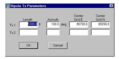
For tensor surveys, configuration information for two transmitters may be stored sequentially in \*.MDE files.
