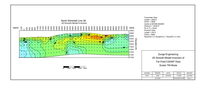
Resistivity inversion results from SCSDEMO plotted with MODSECT, GS Scripter and Surfer for Windows v6.0. The low-resistivity layer tracks a supergene enrichment zone.
