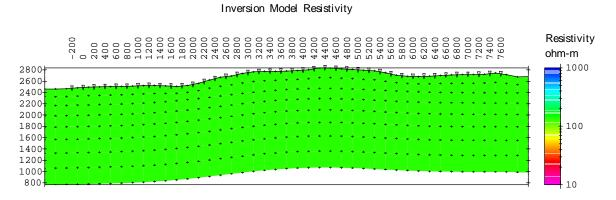
New model section built using data from SCS2DEMO.AVG, SCS2DEMO.MDE and SCS2DEMO.STN with the lowest far-field frequency set to 256 hertz, eight rows of model pixels and a uniform background resistivity.
