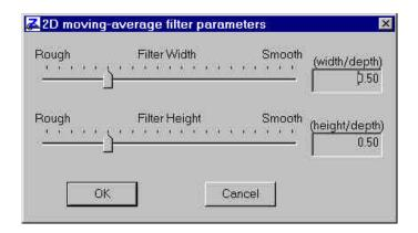
2d moving averages use a low-pass filter which increases in size with increasing model-section-pixel depth. Filter width and height are proportional to model-section pixel depth and the two constants of proportionality may be varied. Widening the filter increases its smoothing effect.
