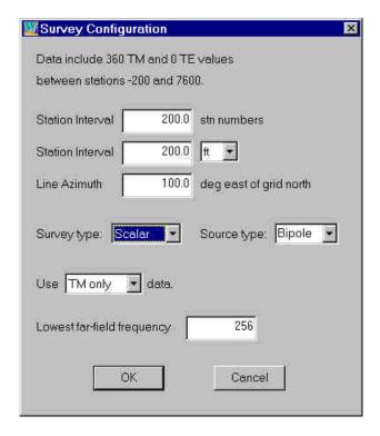
SCS2DEMO.AVG holds TM-mode scalar CSAMT data collected with 200 foot dipoles. Station numbers are distance along line in feet, so both the station interval and the station-interval length are 200. A station interval of 100 and a station-interval length of 100 feet could be used for more detailed modeling. These controlled source data were collected using a grounded bipole source placed 16000 feet north of line 28. The lowest far-field frequency in SCS2DEMO.AVG is 256 hertz.
