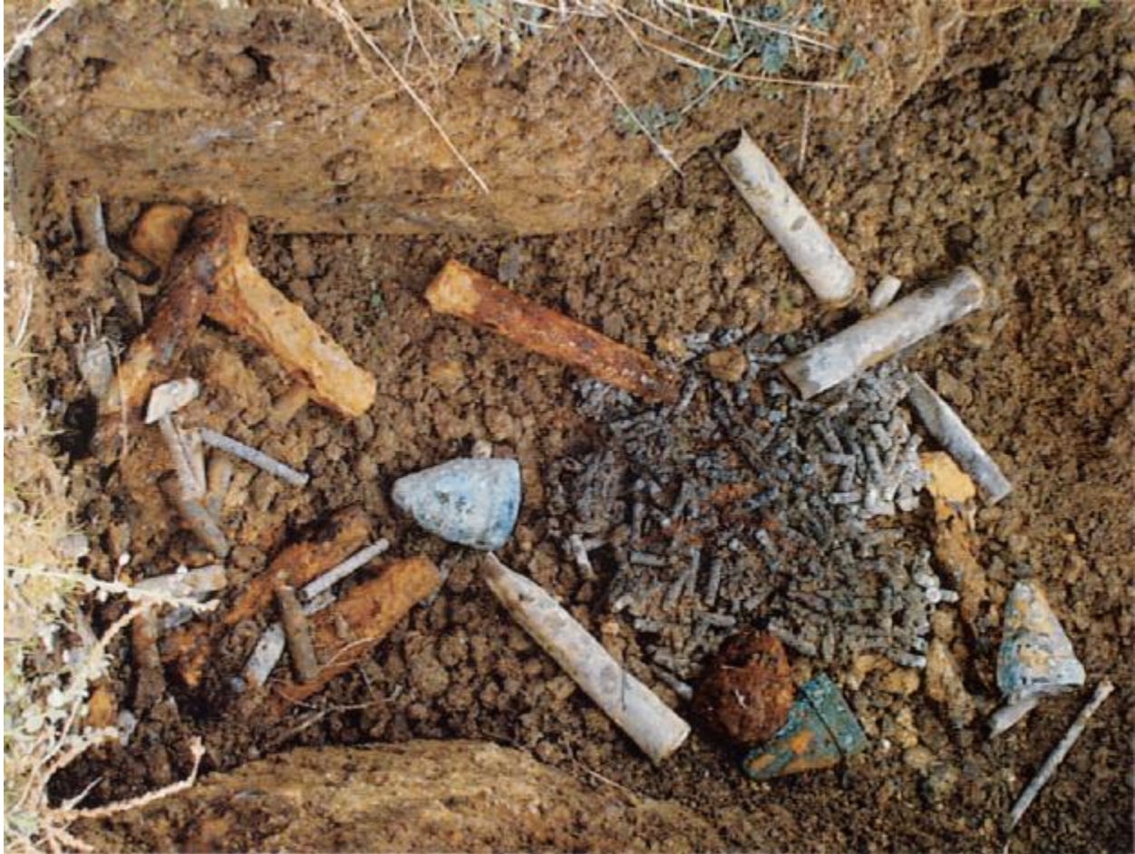
Figure 3. Mass of UXO buried at the test site. A backhoe was used to dig the pit about 1 m deep and compact the backfill.
